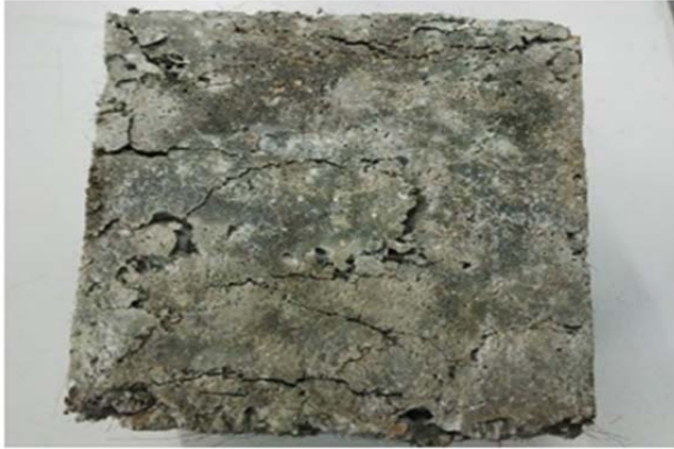
Fig. 4: FRC Cube Sample in Crack Propagation
